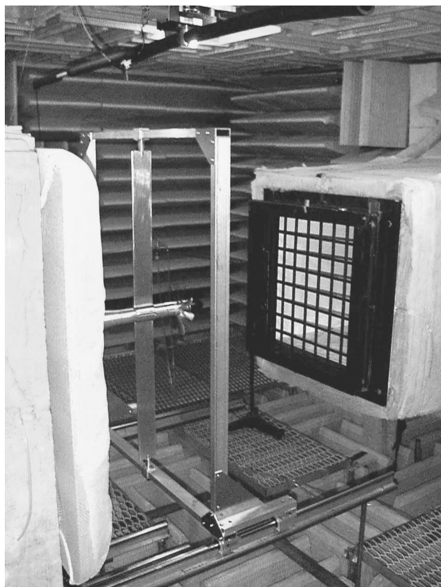
Fig. 3 Propeller/stator test rig mounted in Anechoic Wind Tunnel.
